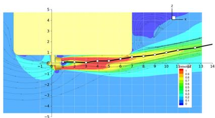
Figure 1: Thruster wake comparison between PIV experiments (black line) and the velocity field obtained from CFD (colour) for a thruster under a barge.
