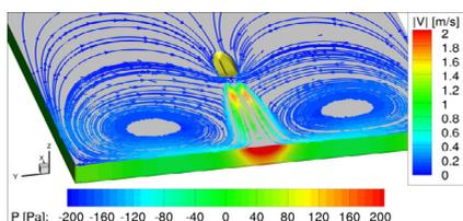
Figure 4: Flow at the free surface due to the thrusters in a confined water area, and the pressure on the quay. The flow shows two clear recirculation areas.
