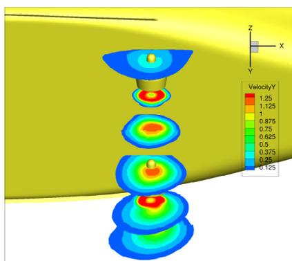
Figure 3: Thruster-thruster interaction for different CFD methods compared to experimental data (top) and the stream wise velocity for one thruster angle.
